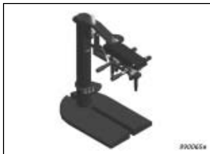
Fig. 7 Alignment jig with handset cradle
